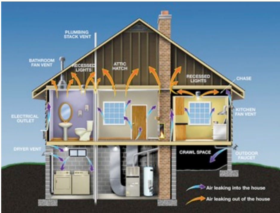
Energy Leakage Points In An Inefficient Home
